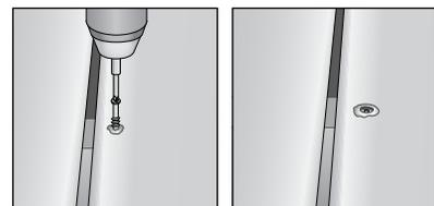
Using your thumb, lightly push the displaced decking material over the hole left by the trim head screw.
