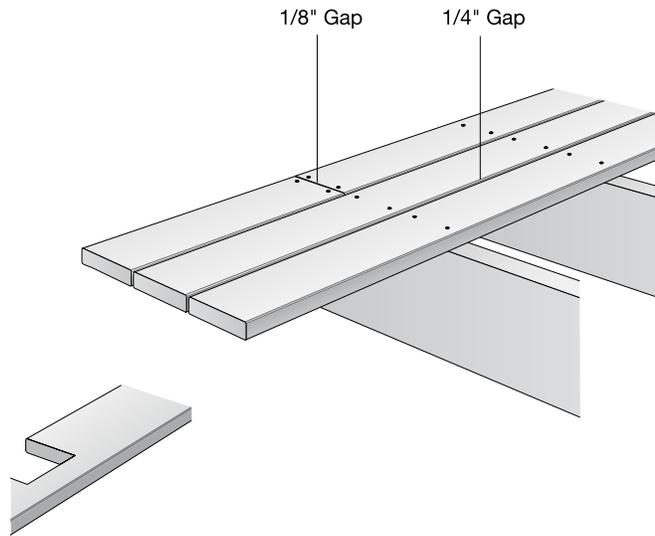
**C.** Staggering the butt joints on long decks usually improves the overall appearance of the finished deck. Some people also prefer a distinctive pattern for the deck boards. To achieve an interesting design, install a pattern board, which eliminates butt joints.
