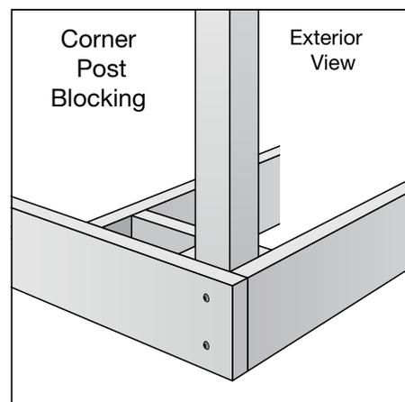
Bolt positions: The top bolt to be no more than 3-inches below the finished deck surface and the bolt spacing to be no less than 4-inches on-center.
