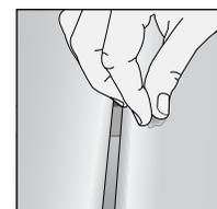
Tap with a hammer, this will cover the trim head screw with decking material.
